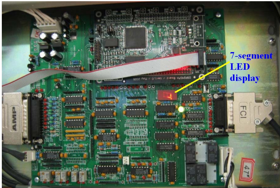
Fig. 5 Seven-segment LED display mounted on interface board
